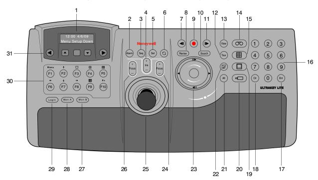
Figure 2-1 UltraKey Lite Controller Keyboard Layout
